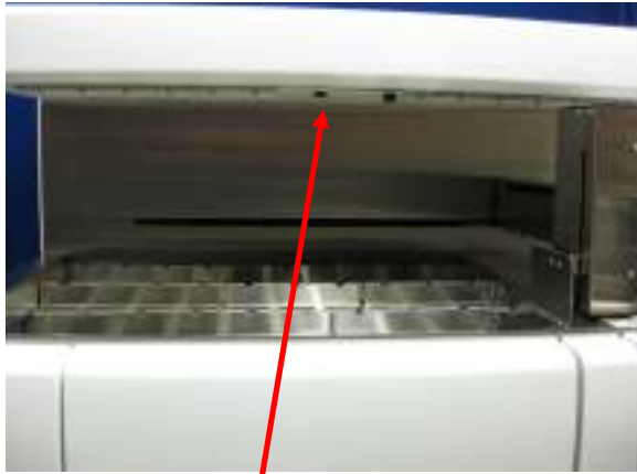
Push button to release the bezel
