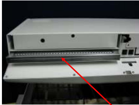
Charcoal Filter behind the bezel
